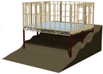
Wall frames installed
