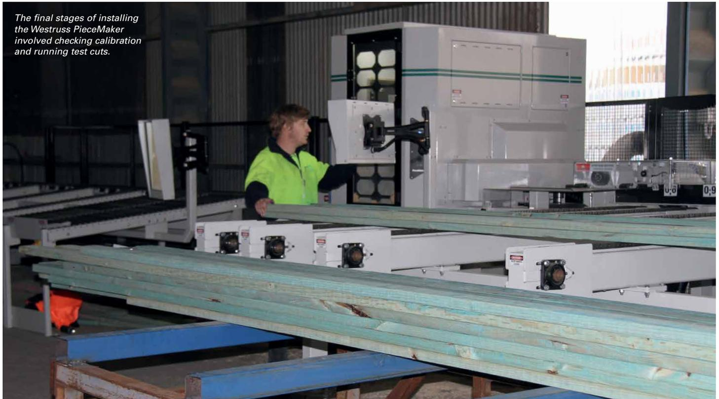
The final stages of installing the Westruss PieceMaker involved checking calibration and running test cuts.
