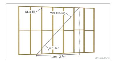
0.8kN/m Bracing Capacity as per AS1684-2010 Residential Timber-Framed Construction, Table 8.18(a)
