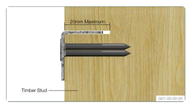
The maximum depth of a notch or saw-cut shall NOT exceed 20mm.
