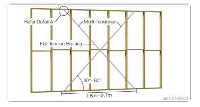
No Stud Ties required for 1.5kN/m Bracing Capacity as per AS1684 Residential Timber-Framed Construction, Table 8.18(b)
