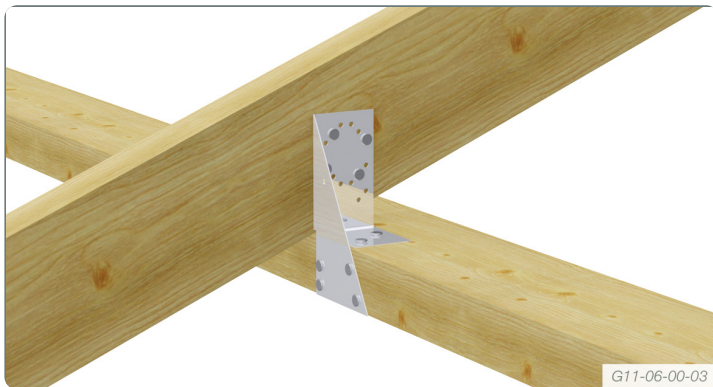
Connecting of Rafters to Wall Plate
