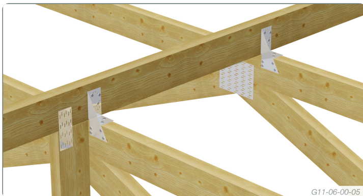
Jack flyovers to truncated truss
