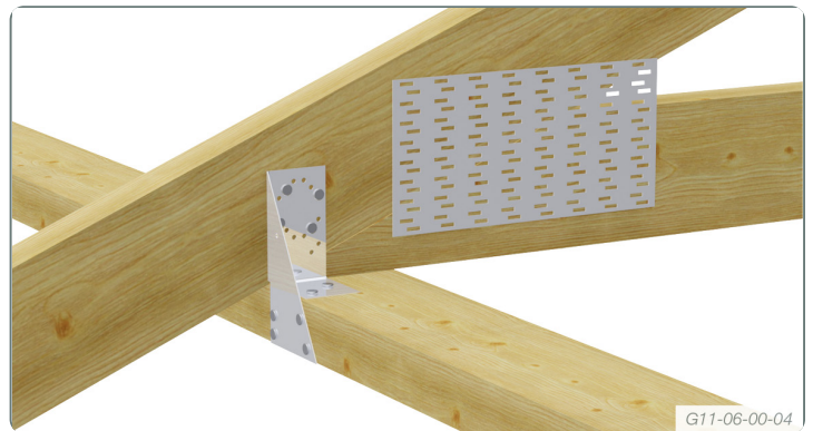
Connecting of Roof Trusses to Wall Plate
