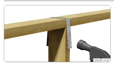
Multinail also manufactures the Nail/Press Stud Tie for easy on-site application. To install, hammer teeth into one side and 3/2.8Ø Multinail nails into the other side.
