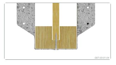
Multinail recommends fixing 30mm-No.6 Type 17 bugle head screw through the I Beam Hanger bottom hole to joist bottom plate.
