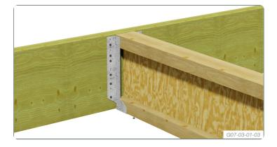
Multinail Face Mounted I Beam Hanger secured full height of I-Joist to beam/bearer using galvanised nails.
