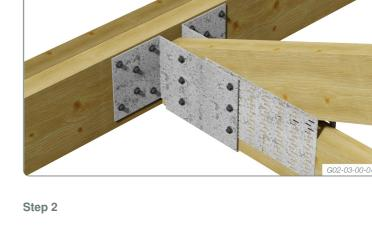
Fix 12/25mm Black Tip #14 screws (6 per side) to the supported truss to ensure that the uplift and anti-rotation features of the Girder Bracket is maintained.
