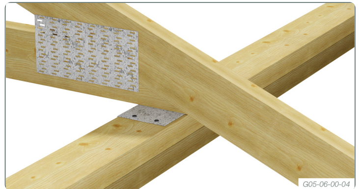
Connecting Roof Trusses to Wall Plates
