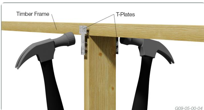
A single Multinail T-Plate can also be hammered into both sides of the frame, allowing flexibility on-site.
