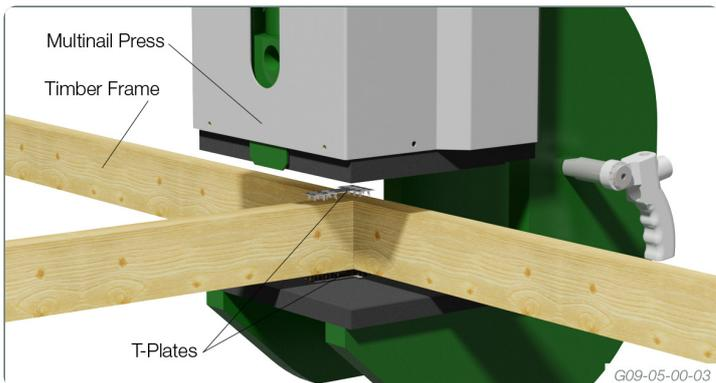
A single Multinail T-Plate is usually positioned on both sides of the frame and then mechanically pressed with a Multinail Press. The Multinail T-Plate is factory pressed to produce a positive, lasting connection.
