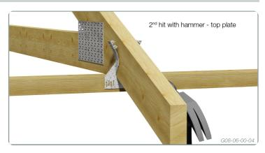
2. Hit the other side of the Quad Grip on top plate (wall). You are now ready to embed Quad Grip into the rafter or truss.
