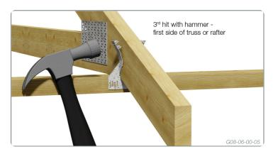
3. One hit on the top left hand side of Quad Grip will embed the teeth into the timber rafter or truss.
