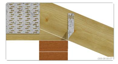
Quad Grips can be used effectively with single or double top plates.
