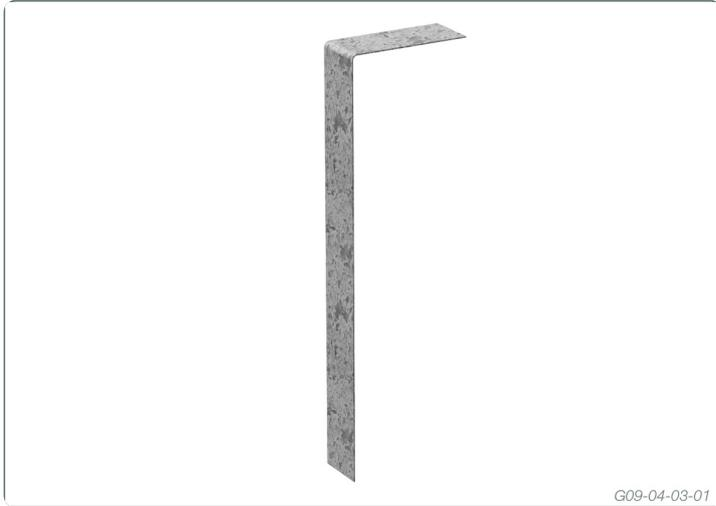
Formed galvanised steel connector designed to provide an effective means of fastening top and bottom wall plates to studs in high wind areas
