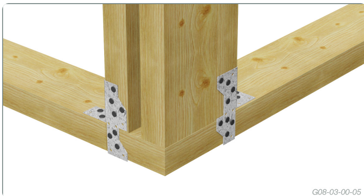
Studs to bottom plates
