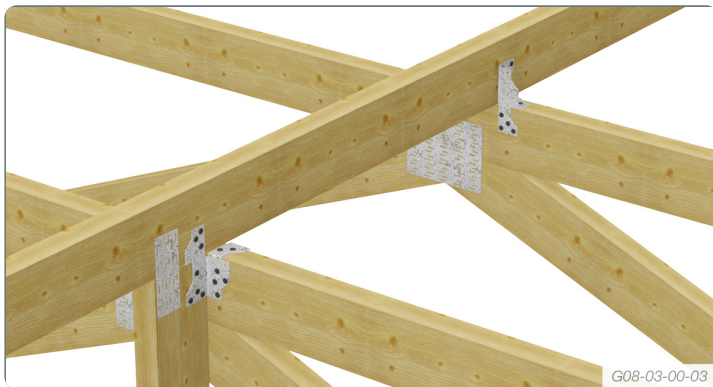
Jack flyovers to truncated truss
