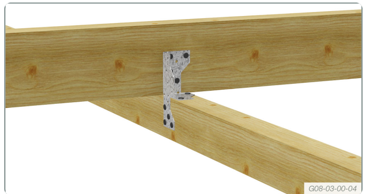
Ceiling joist to hanging beam
